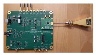
Figure 2: HMC6300 TX front-end fitted with SAGE horn antenna.
