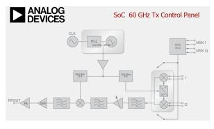
Figure 1: Block diagram of the HMC6300 SoC.
