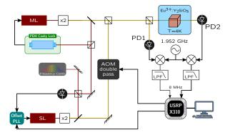
Figure 1: Schematics of the experimental setup. The GNU Radio flowgraph is driving the USRP to generate multi frequency signal for AOM and computing the correction applied to the offset of the PLL from the two RX signals
