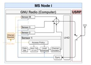
Fig. 4. EPHYL MS Node Block Diagram
